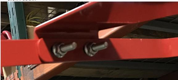
12) Last step would be to adjust the two front guard components as needed, for safety. After that is complete, go around and assure all hardware is tightened properly.
