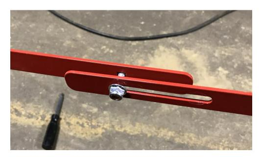
8) Next remove the two nuts under the throwing plate that mount to the frame as shown below.
